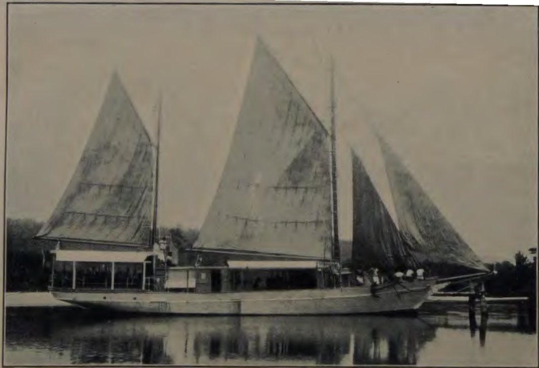
MISSION SHIP "EVANGEL" SOUTH SEA EVANGELICAL MISSION, SOLOMON ISLANDS 50 Tons Gross. 45 H.P. Crude Oil Engine. Speed 7 knots
